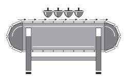
up to 203.2 mm (3.5" up to 8"). Application field: Multi-colour printing up to 16 colours, for medium-sized to large articles; ideal for interlinked systems of many machines.
