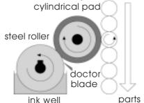
cylindrical die plate. The cylindrical die plate is rotated in the ink tray. The stationary doctor blade "cuts" the surplus off the die plate surface. The counter-turning cylindrical printing pad picks up the ink and transfers it onto the parts.
