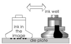
larger, as the ink cup needs a park position. All manufacturers are currently trying to improve this system. The only real problem is that through normal daily use, the ink works its way out of the bottom of the cup.
