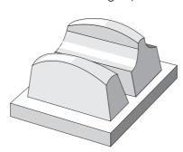
(aluminium or wooden panel). Furthermore, existing pads can be shortened or cut which is one way to adapt existing pads to special printing applications. When moulding the pad a hollow space can be included which will affect the ductility of the pad. If the printing result is still not satisfactory, a special pad shape will have to be produced as mentioned
