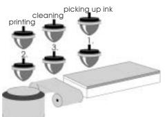
came from the industrial users of pad printing. Much has been done by the manufacturers in the past few years. The pads of single or multi-colour machines are cleaned by adhesive tape. When the pad prints onto the adhesive tape during production, it is cleaned effectively and carefully by the adhesion of the tape. The dirty tape is then automatically advanced. This
