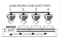
can be added. The economical quantity of printed parts for a shuttle ranges from 5,000 to 30,000 parts/print run. Quantities over 50,000 parts/print run can be achieved more economically with a conveyor.
