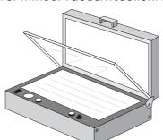
die plates should only be removed in a darkroom with yellow or red light or in a room with subdued light, otherwise exposure faults are possible. The repro film is put at the exact position on the print plate, face up with text readable, and pressed down on the print plate by either the glass pane or the vacuum foil of the
