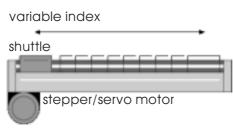
of the shuttles is variable, several machines can be interlinked with one shuttle.
