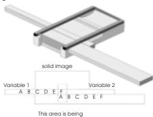
together and can be moved against each other in the ink tray. Because of this sliding, numerous number/digit combinations can be printed, without having to stop the printing process for a long time. In combination with steel plates, the customer's logo can be printed alongside. This application has been accepted mostly in the industrial sector.
