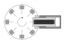
part carriers. Because the mass which is moved is quite large, the indexing time is longer on rotary tables than with conveyors.
