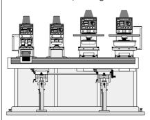
for such an interlinked system, one large 4-colour stand-alone machine can be linked with a 2-colour table-top model, a single-colour in-line machine and a single-colour in-line swivel-head machine, all combined at a large linear conveyor. One machine works as a pulse generator. This means all control functions are generated from its control board.
