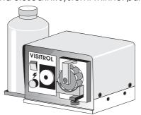
timing, single drops of thinner are automatically added to the ink system. For good results, tests have to be made during one shift, for example, to find the optimum dosage.
